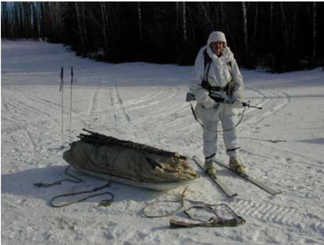
Fig. 18-8. The akhio is a fiberglass sled designed to carry up to 200 lb of equipment. Infantry squads usually use them to carry their 10-man tent, stove, fuel, water, and other equipment. The sled weighs 38 lb and measures 88 x 24 x 8 in. Three rails on the bottom help the sled track in a straight line. Maneuvering the fully loaded akhio requires the coordinated efforts of up to four individuals, especially on turns. A knotted rope, seen in this photograph, is placed beneath the akhio as a brake for downhill runs. Photograph: Courtesy of US Army Northern Warfare Training Center, Fort Greeley, Alaska.
