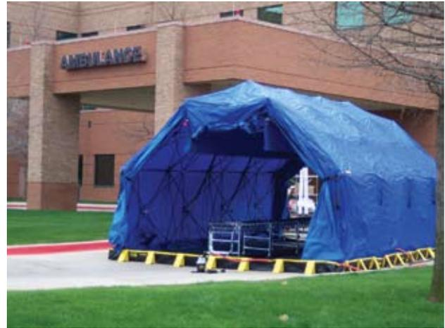
**Fig. 16-6.** A medium sized Reeves DRASH (deployable rapid assembly shelter). The scissors construction allows for tent expansion similar to the TVI tent but with the framework on the inside of the shelter. It also has integrated plumbing and a litter roller system. Can be configured for both ambulatory and litter patients.
