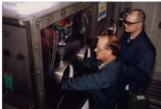
Fig. 18-2. Two chemical agent operators wear Level C protective clothing and use a glovebox as they drain mustard agent from ton containers in the neutralization process at the Aberdeen Chemical and Biological Agent Disposal Facility. Photograph: Courtesy of US Army Chemical Materials Agency, Aberdeen Proving Ground, Md. Available at http://www.cma.army.mil/multimedialogallery . Accessed December 2005.
