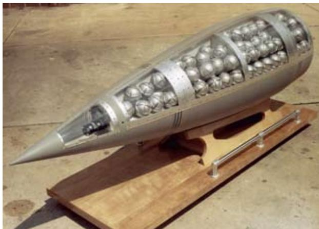
**Fig. 4-12.** A chemical warhead for the Honest John rocket. It was designed to break apart and disperse the spherical bomblets of nerve agent.
