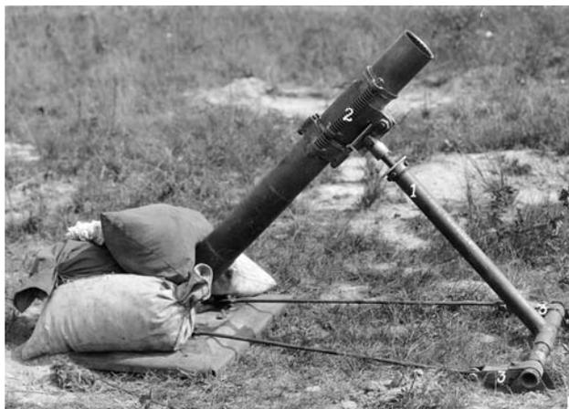
**Fig. 4-7.** An experimental 4.2-in chemical mortar, showing (1) the standard, (2) the barrel with the shock-absorbing mechanism, and (3) the tie rods connecting the standard to the baseplate. This weapon differed from the Stokes mortar, its predecessor, in that it was easier to set up and it was rifled; the spiral grooves can be seen on the inside of the barrel at its muzzle.
