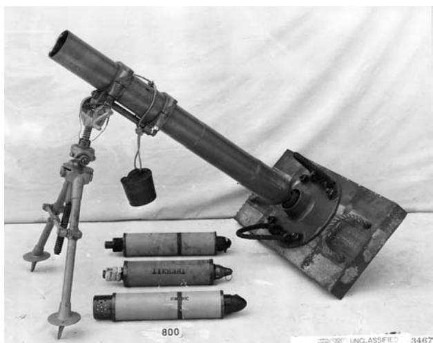
**Fig. 4-6.** A complete Stokes mortar with ammunition and accessories for firing.
